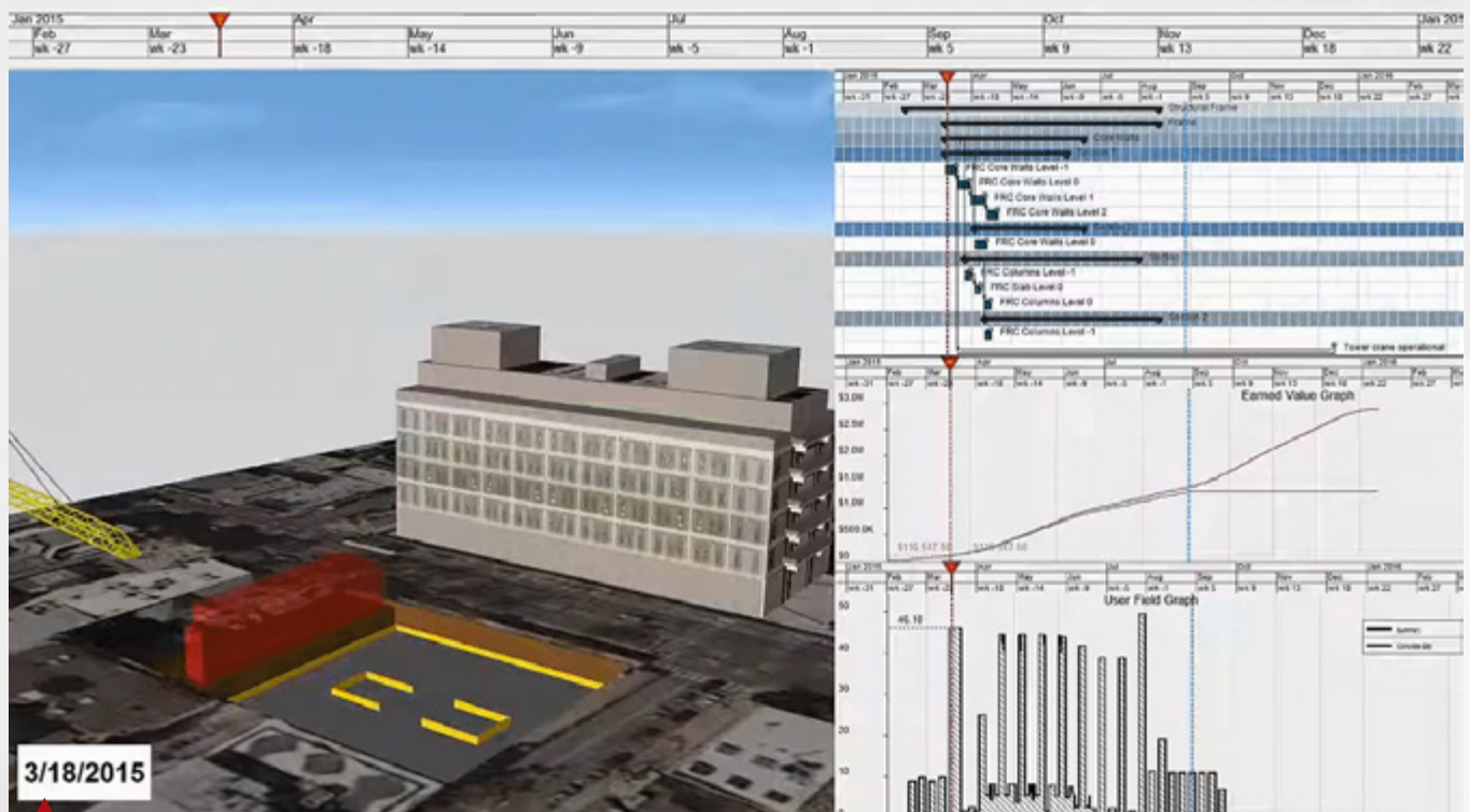
Example Output from SYNCHRO Pro 2016 demonstrates how to combine schedule, cost, and material tracking with construction sequence visualization
