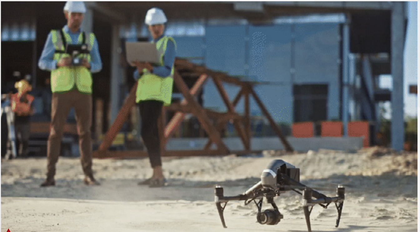
High-resolution drone images are turned into a reality mesh linked to a digital twin for virtual bridge inspection.
